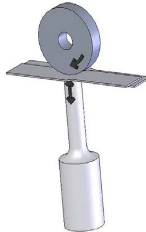
Standing sonotrode and vertically rotating anvil wheel
