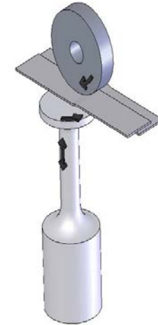
Horizontally rotating sonotrode and vertically rotating anvil wheel
