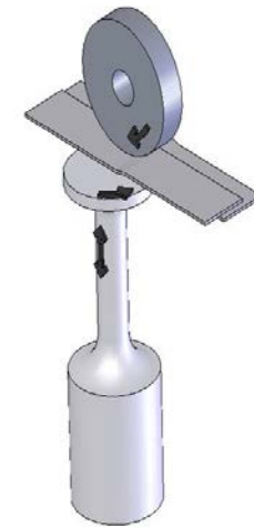
Horizontally rotating sonotrode and vertically rotating anvil wheel
